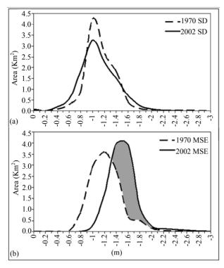
Figure 3. Frequency distributions of specific elevations in 1970 (dotted line) and 2002 (solid line) in SD (a) and MSE (b) sub-areas (see Figure 3). In (b), note shift of mode from -1.1 to -1.60, and increase in areas deeper than -1.4 m.
