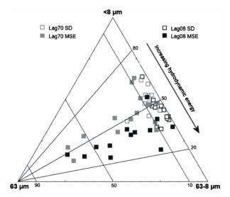
Figure 4. Ternary diagram of surficial sediments based on >63/63 - 8/<8 µm ratios.
