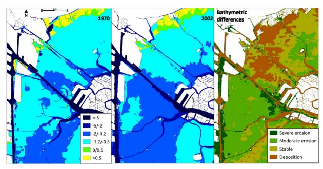
Figure 2. Bathymetric maps of SIN (1970; 2002), with bathymetric data shown in metres (increasing depth shown by progressively darker blue colours). Sedimentation map showing differences between 2002 and 1970. Deposition = differences of >0.1 m, stability = differences of  $\pm 0.1$  m, moderate erosion = differences of between -0.5 and -0.1 m, severe erosion = differences of <-0.5 m.
