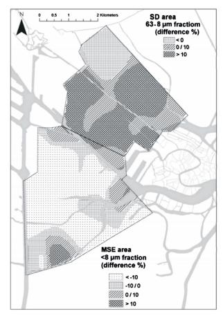
Figure 5. Differences between Lag08 and Lag70 in distribution of 63 - 8  $\mu$ m fraction (SD sub-area) and <8  $\mu$ m fraction (MSE sub-area).
