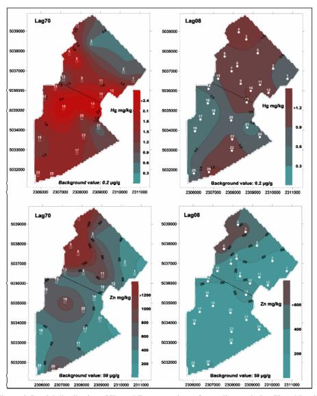
Figure 6. Spatial distribution of Hg and Zn content in surface sediments in Lag70 and Lag08.
