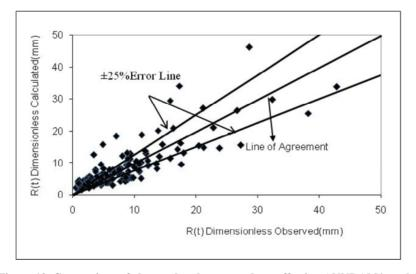
Figure 10. Comparison of observed and computed runoff using ANNDAM1 model
