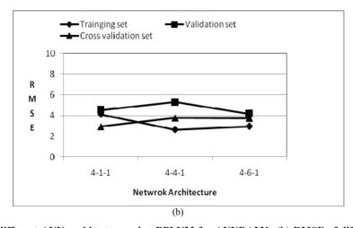
Figure 5. (a) RMSE of different ANN architecture using BPLVM for ANNDAM1; (b) RMSE of different ANN architecture using BPLVM for ANNDAM2
