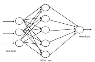
Figure 1. Three layer feed-forward neural network
