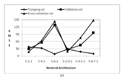
Figure 4. (a) RMSE of different ANN architecture using BPLVM for ANNPAM1; (b) RMSE of different ANN architecture using BPLVM for ANNPAM2; (c) RMSE of different ANN architecture using BPLVM for ANNPAM3; (d) RMSE of different ANN architecture using BPLVM for ANNPAM4; (e) RMSE of different ANN architecture using BPLVM for ANNPAM5
