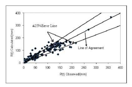
Figure 9. Comparison of observed and computed runoff using ANNPAM4 model
