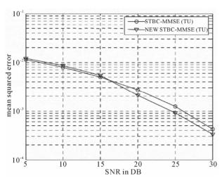
Figure 3. MSE of channel estimators under TU delay profile [8].
