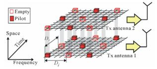
Figure 6. Three dimensional (3D) pilot grid for MIMO-OFDM [14].
