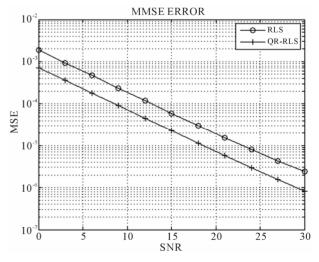
Figure 5. MMSE error for 2 × 2 MIMO system [13].
