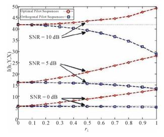
Figure 4. CMI versus  $r_L$  without transmit correlation and receive correlation [11].
