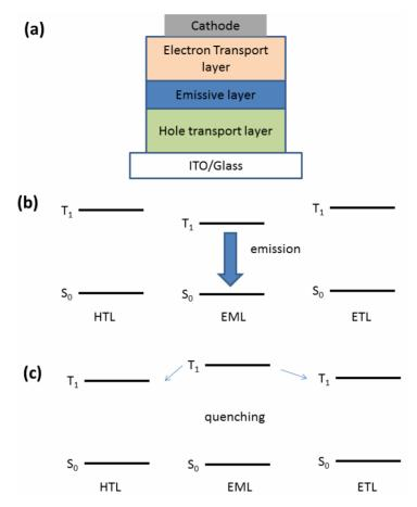
Figure 1. (a) Schematic representation of an simple OLED; (b), (c) The relationship of the relative triplet energies of ETL, HTL and the emitter.
