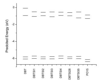
Figure 5. The predicted energy levels of the substituted silanes.
