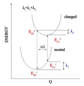
Figure 6. Schematic plot of reorganization energy.
