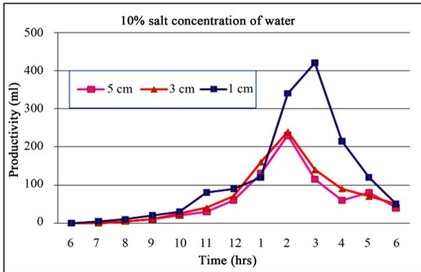
Figure 11. Productivity vs time for various water level.
