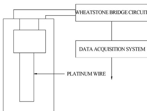
**Figure 5. Thermal conductivity measurement.**
