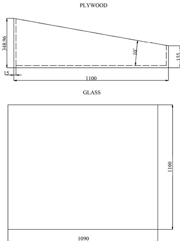
**Figure 2.** Schematic diagram of our solar still.
