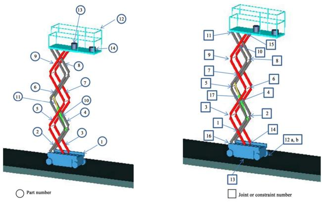
Figure 3. An ADAMS model of the scissor lift.
