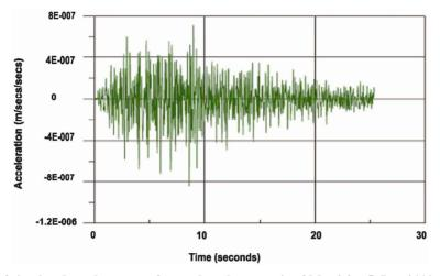
Figure 3. Time history of simulated accelerograms for earthquake scenario of M > 2.9 < 5, R = 466 km on rock characteristic of Nsukka, Eastern Nigeria.
