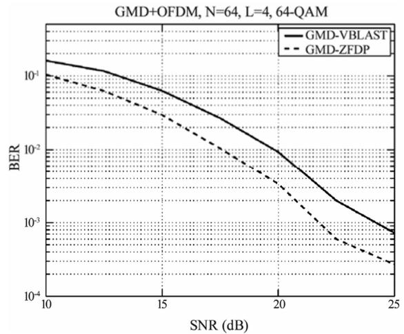
Figure 12. BER performance of GMD based MIMO-OFDM systems [2].
