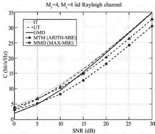
Figure 9. Average capacity for  $4 \times 4$  MIMO configuration [2].
