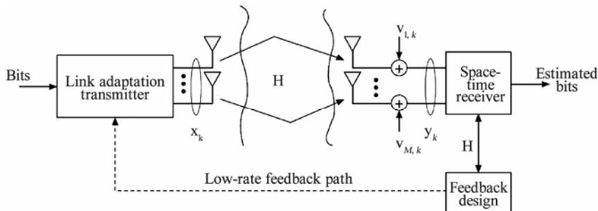
**Figure 17. Limited feedback closed-loop MIMO system [40].**
