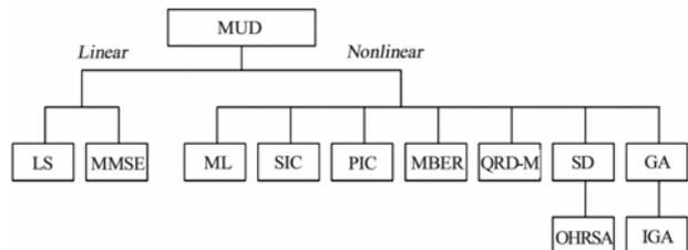
**Figure 26. Various multiuser detectors (MUDs) for MIMO-OFDM systems [3].**
