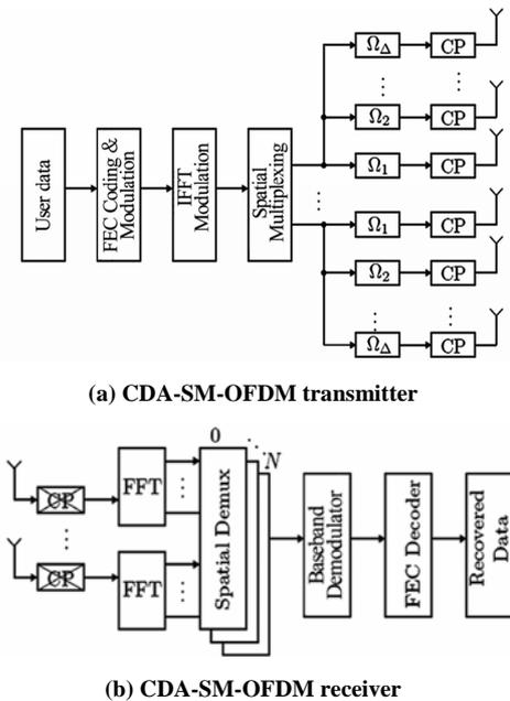
**Figure 3.** CDA-SM-OFDM system transmitter and receiver [35].
