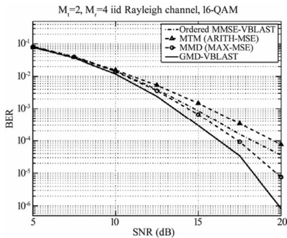
Figure 10. BER performance for  $2 \times 4$  MIMO configuration [2].
