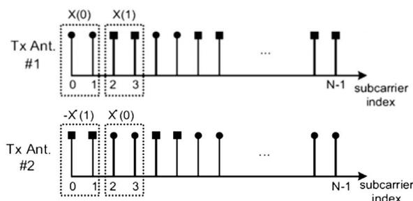
**Figure 23.** Data assignment scheme for ICI reduction in  $2 \times 1$  SFBC-OFDM system [46].
