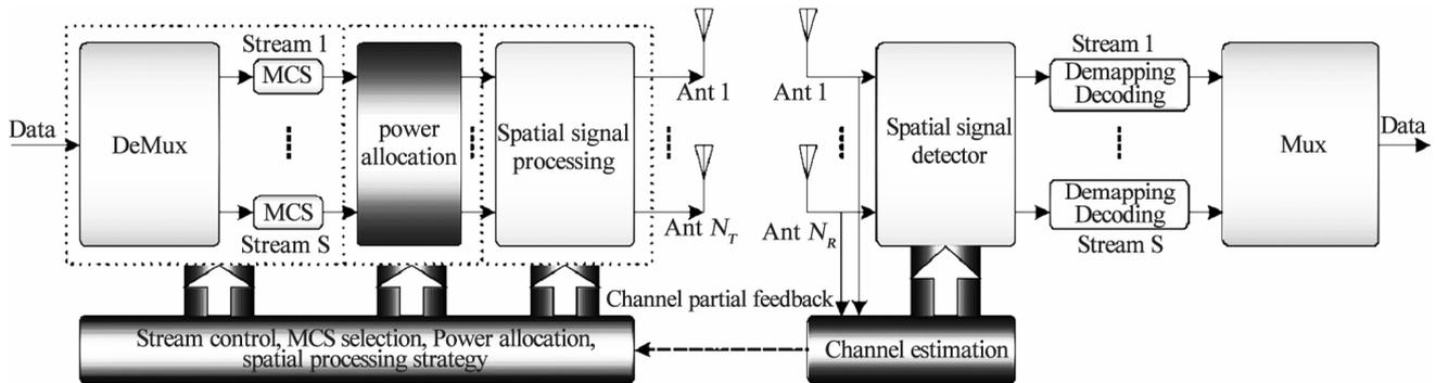
**Figure 20.** MIMO-OFDM system with partial feedback [42].
