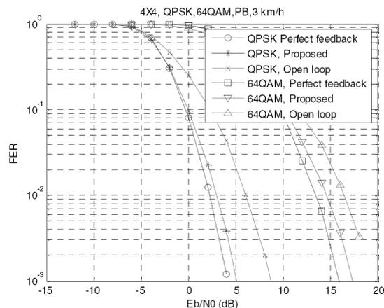
**Figure 22.** FER performance for coded  $4 \times 4$  MIMO configuration [42].
