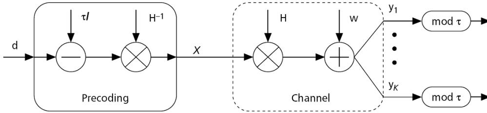
Figure 51. Vector precoding [48].
