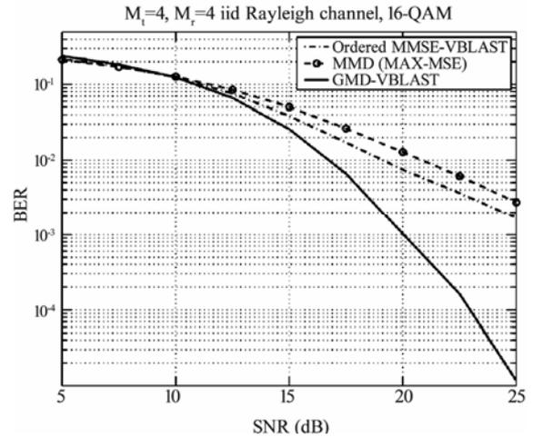
Figure 11. BER performance for  $4 \times 4$  MIMO configuration [2].
