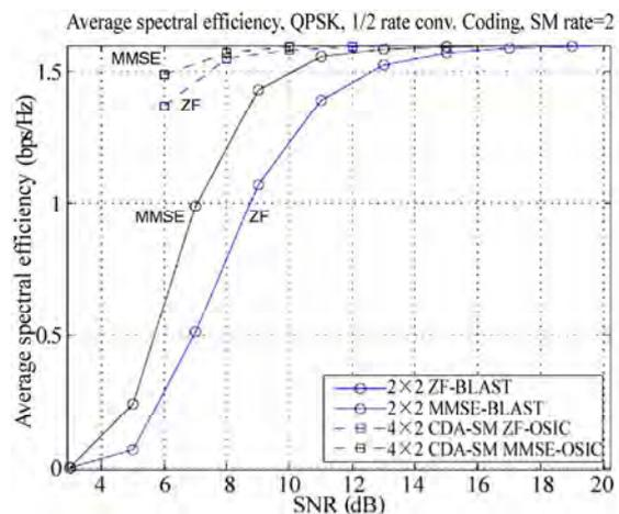
**Figure 5.** Average spectral efficiencies in bps/Hz [35].
