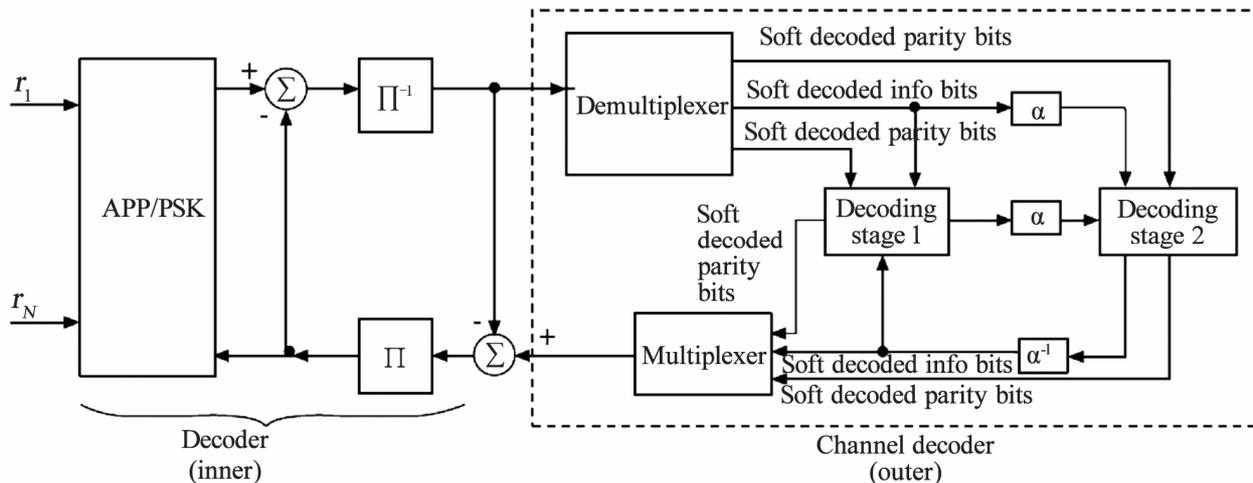
**Figure 14.** Receiver structure for the ST-BICM MIMO system [38].
