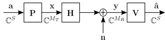
**Figure 50. System model for MU-MIMO downlink transmission [55].**
