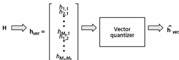
**Figure 18. Channel Quantization [40].**
