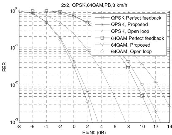
**Figure 21.** FER performance for coded  $2 \times 2$  MIMO configuration [42].
