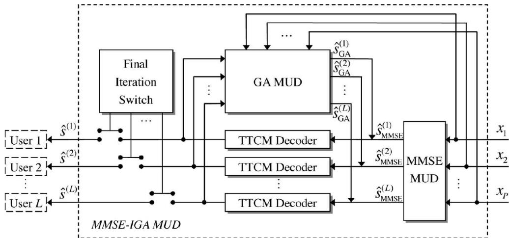
Figure 44. Schematic diagram of an IGA MUD [3].
