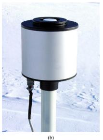
Figure 1. (a) CMP6 pyranometer; (b) NILU-UV irradiance meter.
