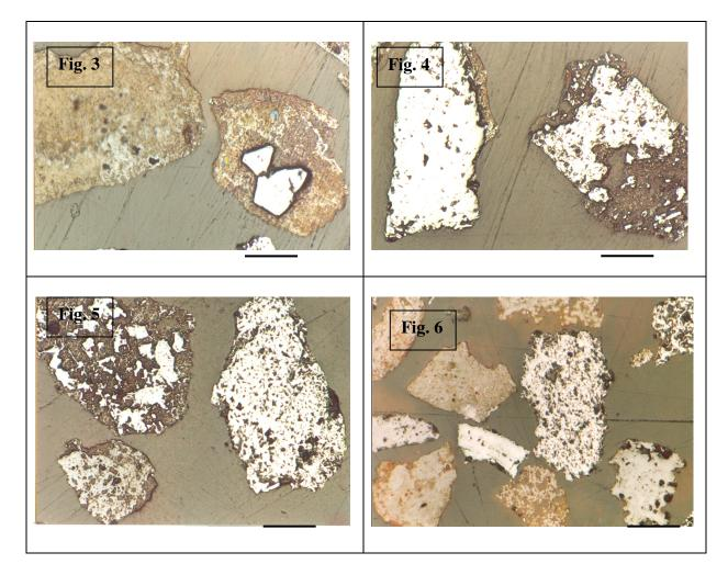
Fig.3: Photomicrograph showing free microporous vitreous goethite and locked martite-ochreous goethite. Scale bar:  $70 \,\mu$ m.
