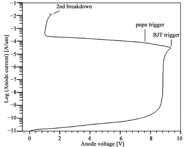
**Figure 4.** Anode I-V characteristics of the `lvtr_thyristor` device.
