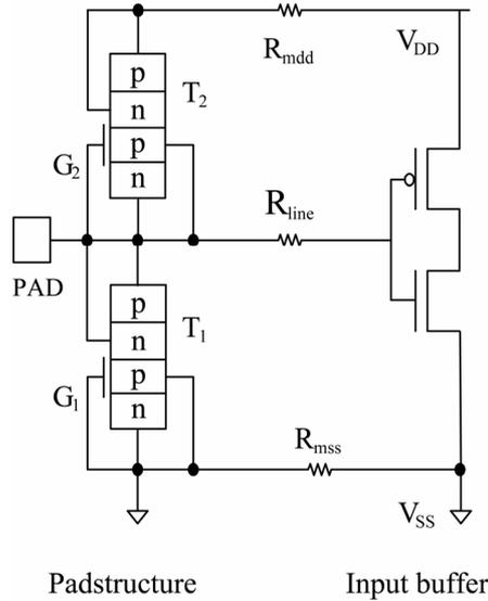
Figure 8. Protection scheme (2) utilizing thyristor devices only.
