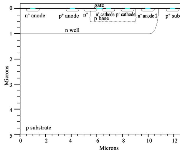
**Figure 5.** Cross section of the diode device.
