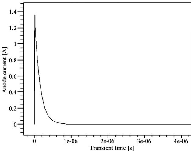
**Figure 12. Variation of the anode current of  $T_1$  in a PS mode when using the protection circuit (1).**
