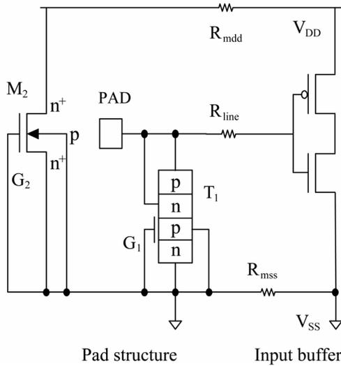
Figure 7. Protection scheme (1) utilizing a thyristor device.
