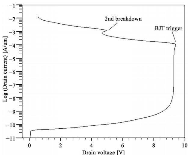
**Figure 2.** Drain I-V characteristics of the NMOS device.
