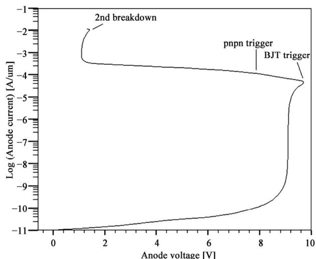
**Figure 6.** Anode current-voltage characteristics of the lvtr\_thyristor\_up device.
