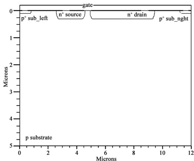
**Figure 1.** Cross section of the NMOS device.
