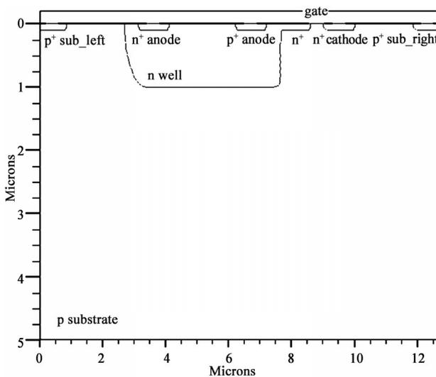
**Figure 3.** Cross section of the `lvtr_thyristor` device.
