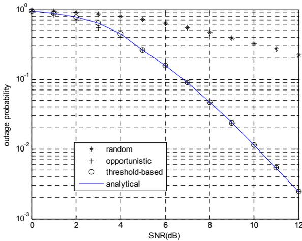
**Figure 2. The outage probabilities of random selection, opportunistic relaying, and threshold-based algorithm without the direct link.**
