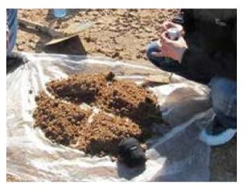
**Figure 2.** Mixing of the samples from the 4 corners to represent one soil sample.
