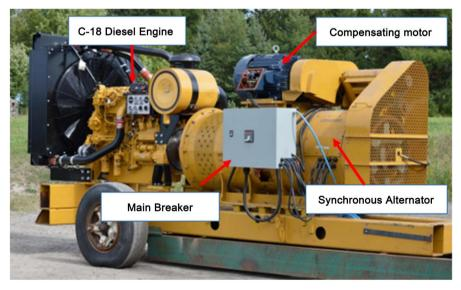
Figure 7. Illustration of the Genset-Synchro GS500X unit with the main components.
