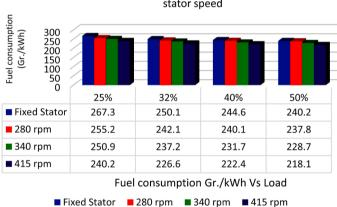
Comparison of the fuel consumption with different stator speed
