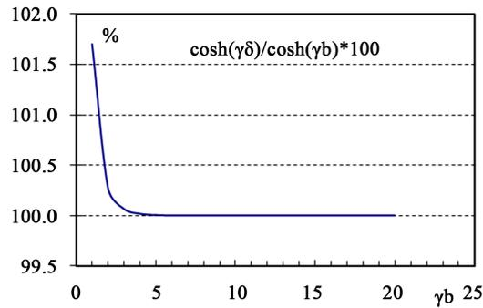
Figure 6. The boundary distance ( $\delta$ ) for  $U_d = 0.99 U_\infty$ .
