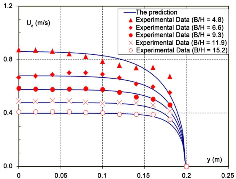
Figure 5.  $U_d$  distributions for the experiments by Atabay [15].
