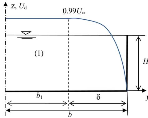
Figure 3. Sketch of half rectangular channel.
