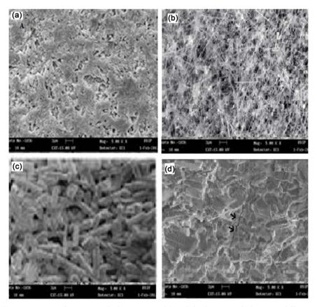
**Figure 3.** SEM ofasa prepared glass-ceramic (a) and for heattreated glasses at different temperatures for 8 hours: (b) 950 °C, (c) 1000 °C, (d) 1100 °C.
