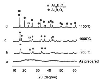
**Figure 2.** XRD patterns (a) for as prepared glass-ceramic, (b) 950 °C, (c) 1000 °C, and (d) 1100 °C.
