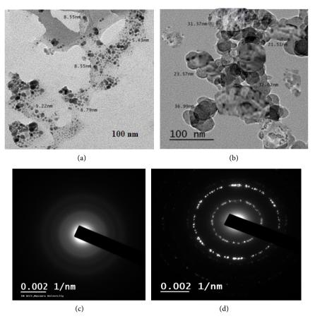
**Figure 4**. TEM of as prepared glass-ceramic (a) and for heat treated glasses at treated at 1100°C (b). EDP of as prepared glass (c) and of glass treated at 1100°C (d).
