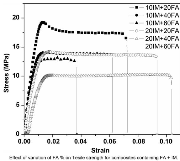
Effect of variation of FA % on Tensile strength for composites containing FA + IM.
