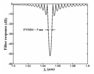
Figure 4. Characteristic response of stop band filter based on ORR.
