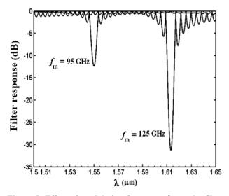
Figure 5. Effect of modulating frequency  $f_m$  on the filter response.
