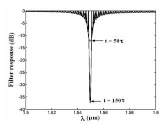
Figure 10. Narrowing of filter response in the resonator loop by increasing the loop delay time.
