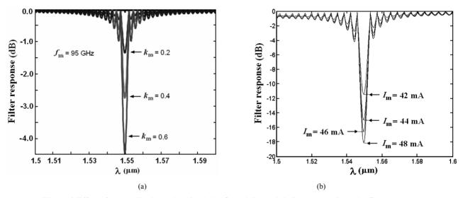
Figure 6. Effect of (a) amplitude modulation index  $k_m$  and (b) modulating current  $I_m$  on the filter response.
