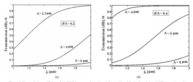
Figure 2. Transmission coefficient of the ORR in terms of wavelength for (a)  $d/\Lambda = 0.2$ , (b)  $d/\Lambda = 0.4$ , and different values of  $\Lambda$ .
