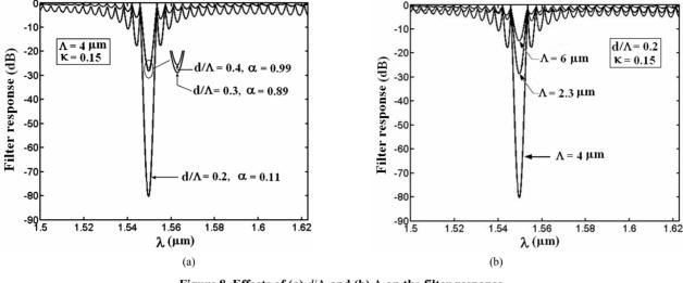
Figure 8. Effects of (a)  $d/\Lambda$  and (b)  $\Lambda$  on the filter response.
