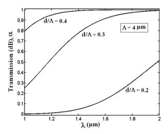
Figure 3. Transmission coefficient of the ORR in terms of wavelength for  $\Lambda = 4\mu m$  and different values of  $d/\Lambda$ .
