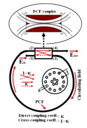
Figure 1. Schematic diagram of an ORR connected to a laser diode at port 1.
