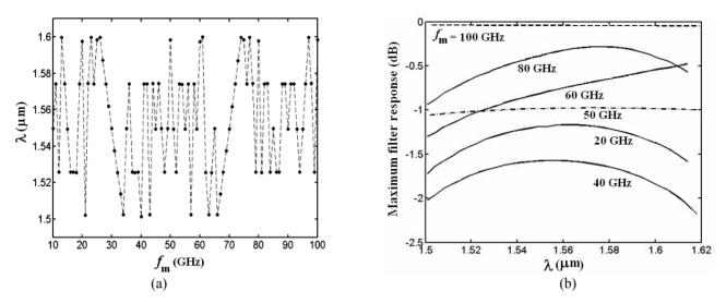
Figure 11. (a) Maximum filter response obtained by the applied modulating frequencies and (b) maximum response versus wavelength for different modulating frequency.
