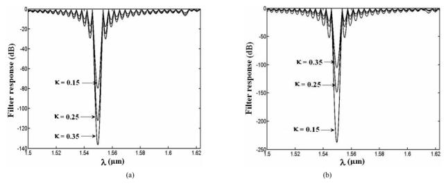
Figure 9. Effect of coupling coefficient  $\kappa$  on the filter response (a)  $d/\Lambda = 0.4$ ,  $\alpha = 0.99$  and (b)  $d/\Lambda = 0.2$  and  $\alpha = 0.11$ .
