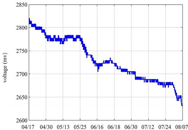
Figure 12. LDAP voltage decay of node battery.
