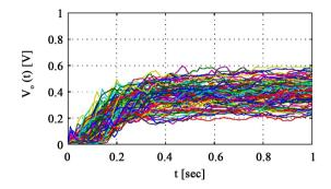
**Figure 6.** Time response of  $V_o$  with the applied force of 9.8 N (100 times).
