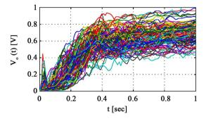
**Figure 7.** Time response of  $V_o$  with the applied force of 14.7 N (100 times).
