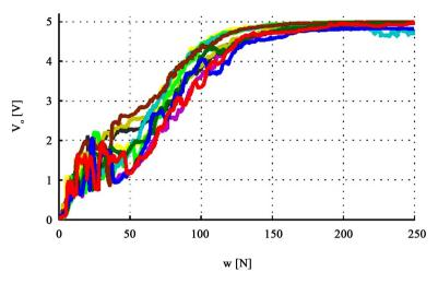
**Figure 5.** The experimentally obtained  $V_o$  variations to the applied force (10 times).
