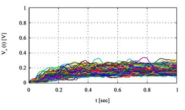
**Figure 4.** Time response of  $V_o$  with the applied force of 4.9 N (100 times).
