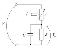
**Figure 3.** A detecting circuit for the rubber sensor *r*. Direct current voltage of 5 V was applied across the terminals (*V* in the figure), and the voltage of  $V_o$  was measured.
