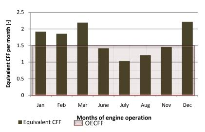
Figure 3. Equivalent creep-fatigue factors for each month of engine operation.
