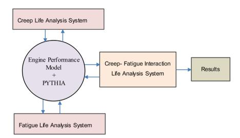
Figure 1. Creep-fatigue interaction analysis system.
