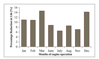
Figure 5. Percentage reduction in life due to fatigue interaction with creep.
