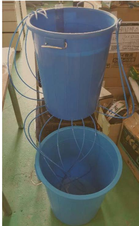
**Figure 1.** Water reservoir (D = 44 cm, H = 43 cm) and 12 releasing holes (ID = 0.4 cm) at the bottom for the response time experiment of potential energy change with reservoir height.
