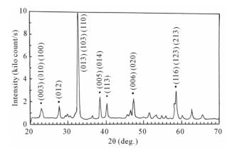
Figure 2. The XRD pattern from YBCO (pressed at 2000 kgf/cm<sup>2</sup>). It was found that any impurity phase decreased to the extent that the sample was almost a single phase.
