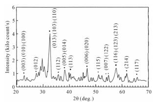
Figure 1. The XRD pattern from YBCO (pressed at 160 kgf/cm<sup>2</sup>). The Millar indices correspond to that of YBCO. The three-peaked structure around 29 degree derived from the impurity phase of  $BaCuO_2$ .
