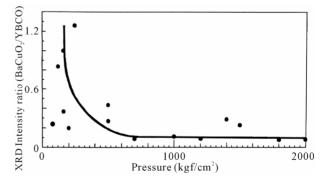
Figure 3. The dependence of the pressure on the intensity ratio of  $BaCuO_2$  to YBCO. Over 700 kgf/cm<sup>2</sup>, The ratio of  $BaCuO_2$  was decreased to the minimum.
