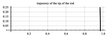
Figure 4. The solid line is the trajectory of the tip of the rod as it falls to the table.
