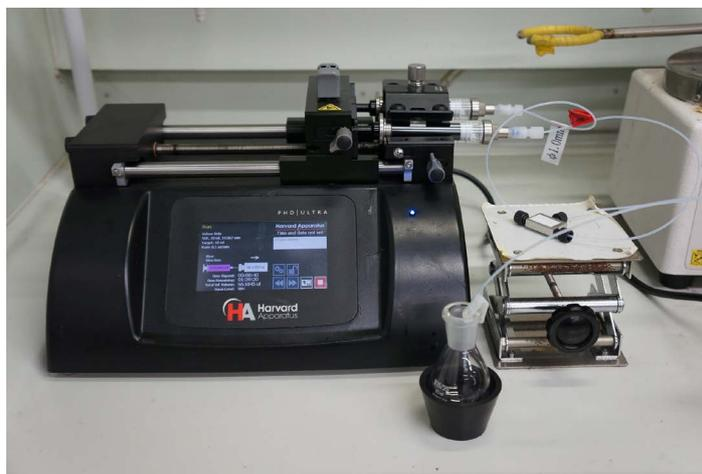
**Figure 1.** Flow system for tetrahydropyranylation.
