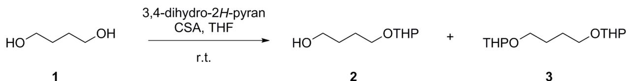
**Figure 2.** Tetrahydropyranylation of 1,4-butanediol (**1**) in a batch reactor.
