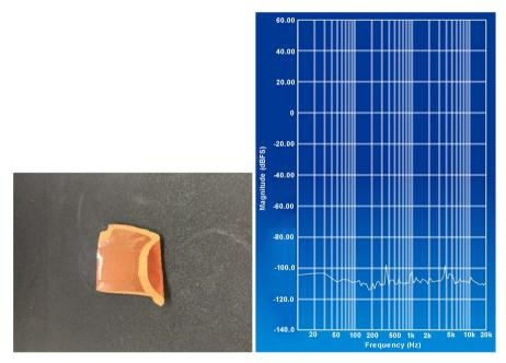
**Figure 4.** (a). A 20th century glazed pottery shard from Mexico; (b) the corresponding vibrational signature, with spikes in the 4K, 1K, and 300 Hz range, and low frequency vibration, with a peak at the 30 Hz range.
