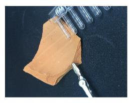
**Figure 2.** The signal source and the accelerometer are placed approximately one inch apart for standardized signal capture.
