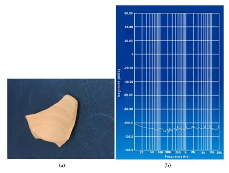
**Figure 3**. (a): A commercially available, common 20th century unglazed, lead-free pottery shard made in Mexico; (b) the corresponding vibrational profile, with spikes in the 9K, 6K, and 1K Hz frequencies, and low frequency vibration in the below 10 Hz range.
