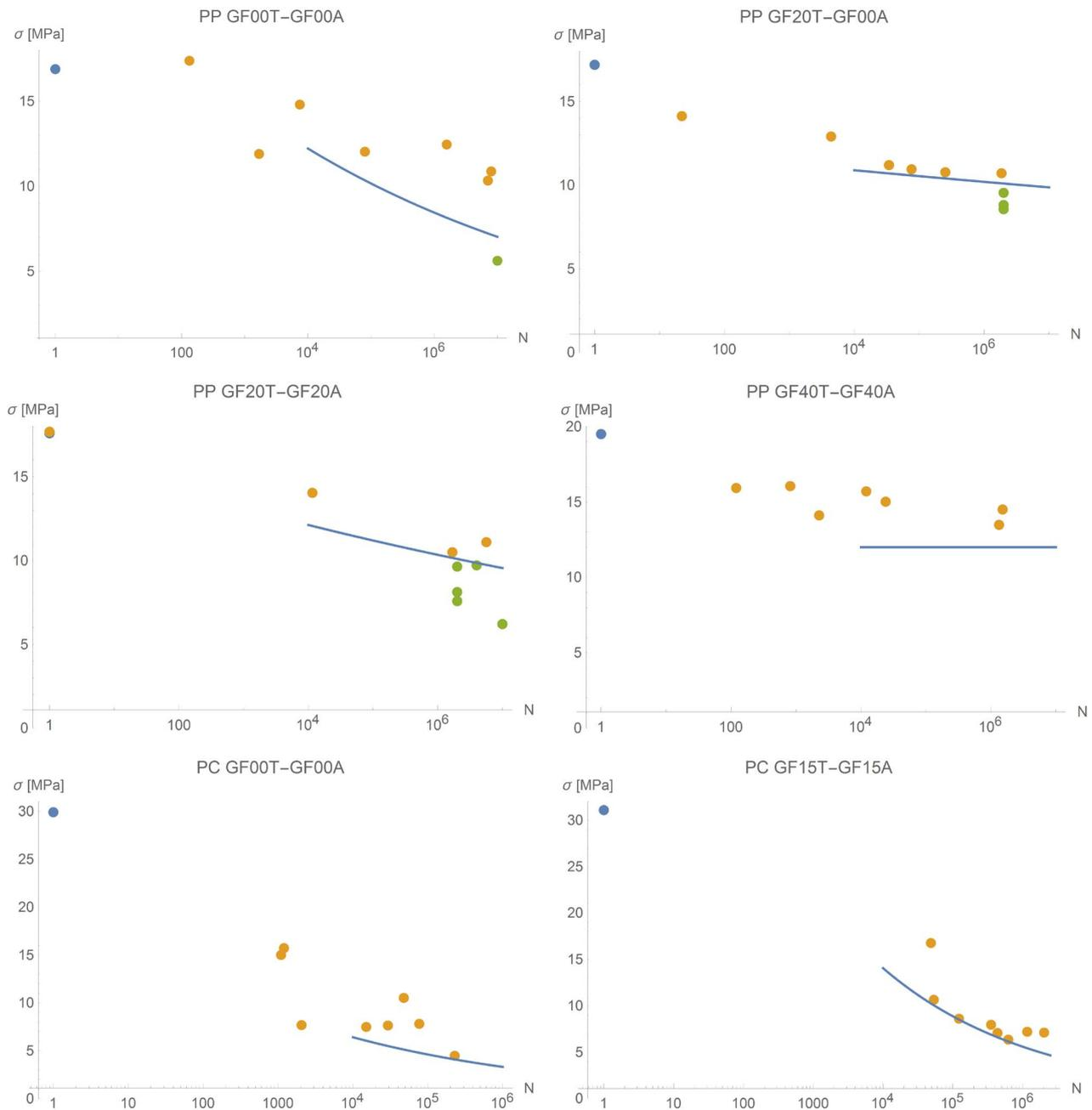
**Figure 4.** S-N curves of PP (four upper graphs) and PC (two lower graphs) composite weld joints for cyclic shear loading with stress ratio  $R = 0.1$ . Orange points mean the moment of the specimens rupture, green points mean the moment when the test was ended and the weld area measured, green points mean static strength of the weld joint.
