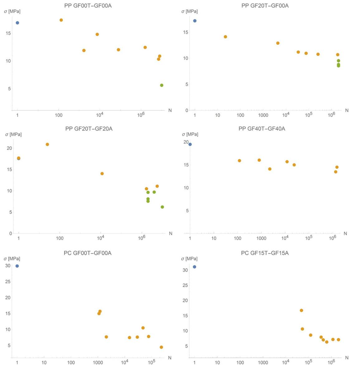
**Figure 3.** Weld joint stress at specimens rupture after  $N$  cycles (orange), stress of intact specimen after the stopping the test (green) and static strength of weld joints (blue) for selected sets of material combinations. Four upper graphs relate to PP reinforced composites and two lower graphs relate to PC reinforced composites.
