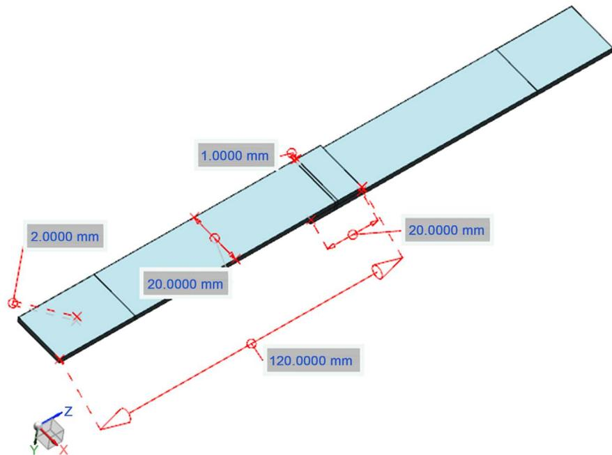
**Figure 1.** The scheme of welded materials for shear test.
