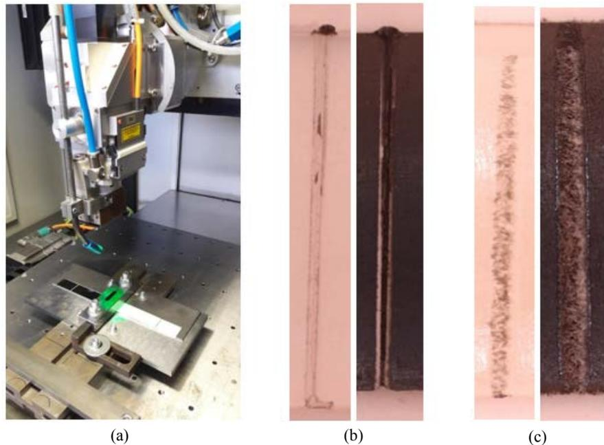
**Figure 2.** Laser station with specimen attached in the tool ready to welding process (letter a), examples of separated parts of welded specimens after the static test under the microscope for PP GF00T-GF00A (letter b) and GF20T-GF40A (letter c) are on the right.
