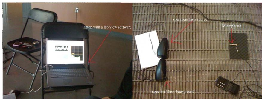
**Figure 4.** Test setup including (the speakers, the microphone, and the software) in the anechoic chamber.
