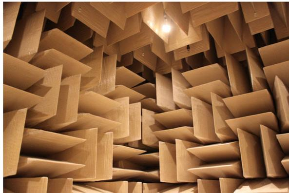
**Figure 1.** Side of the anechoic chamber in which the experiment took place.
