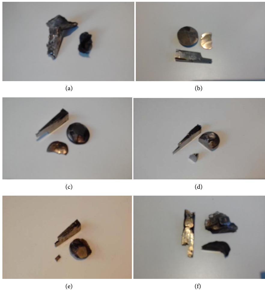
Figure 2. Pictures of different cast wedges of Zr based BMGMC made from vacuum arc melting and Cu mold suction casting. (a) \text{Zr}_{47.5}\text{Cu}_{45.5}\text{Al}_5\text{Co}_2 alloy without inoculants (miss run); (b) \text{Zr}_{47.5}\text{Cu}_{45.5}\text{Al}_5\text{Co}_2 without inoculants (proper riser); (c) \text{Zr}_{47.5}\text{Cu}_{45.5}\text{Al}_5\text{Co}_2 without inoculants (another view); (d) \text{Zr}_{65}\text{Cu}_{15}\text{Al}_{10}\text{Ni}_{10} without inoculants; (e) \text{Zr}_{47.5}\text{Cu}_{45.5}\text{Al}_5\text{Co}_2 (with 0.25 wt.% inoculant 1); (f) \text{Zr}_{47.5}\text{Cu}_{45.5}\text{Al}_5\text{Co}_2 (with 0.50 wt.% inoculant 1).
