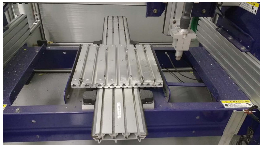
Figure 2. Large slotted table with mechanical screw clamps for securing specimens.
