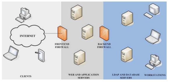
Figure 1. Standard enterprise network configuration [2].
