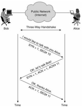
Figure 4. Basic TCP three-way handshake [14].
