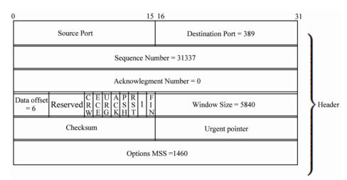
Figure 6. TCP Header-modified for connections with LDAP servers.
