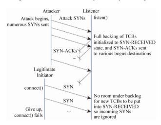
Figure 5. Basic SYN flooding attack [16].
