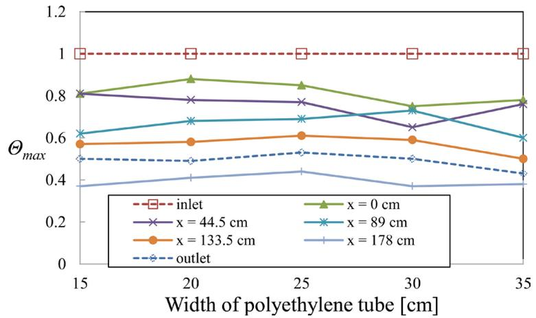
**Figure 14.** Relationship between  $\Theta_{max}$  and  $W_p$  with air injection.
