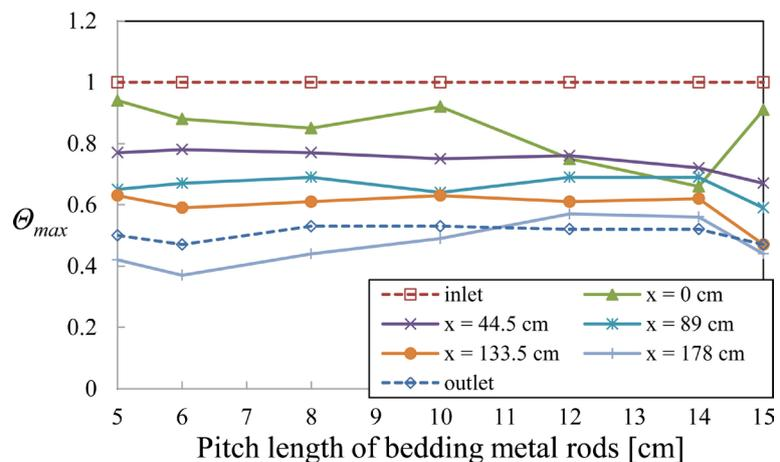
**Figure 11.** Relationship between  $\Theta_{\max}$  and  $X_p$  with air injection.
