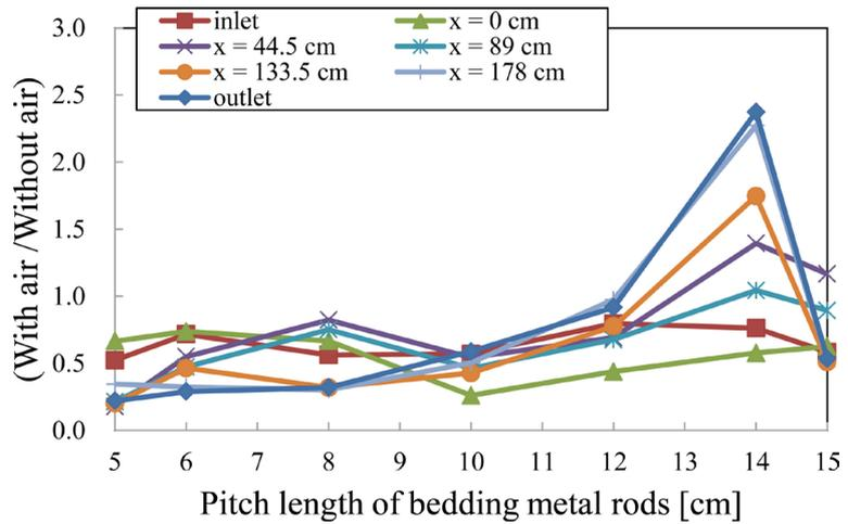
Figure 13. Comparison of time required to reach steady state in all conditions with and without air injection.
