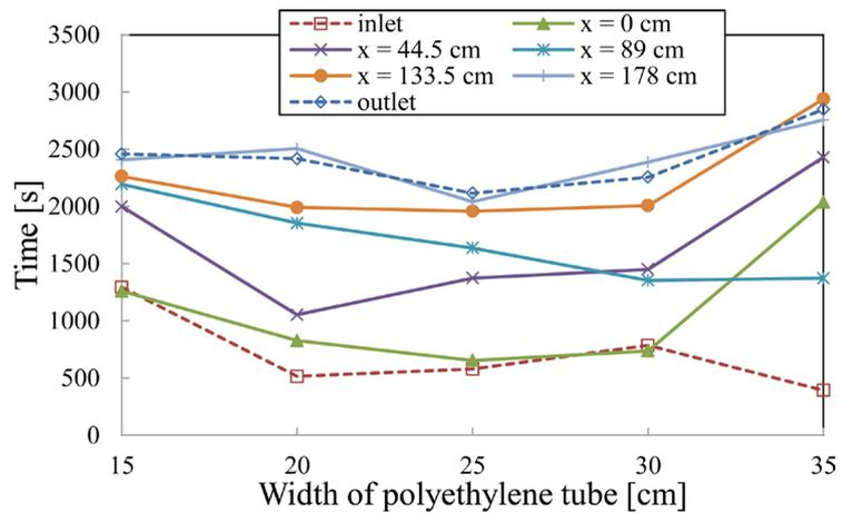
**Figure 15.** Relationship between time required to reach steady state and  $W_p$  with air injection.
