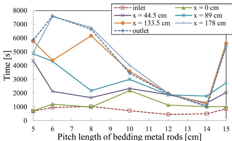
**Figure 8.** Relationship between time required to reach steady state and  $X_p$
