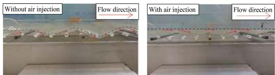
**Figure 10.** Appearance of flow condition (L: without air injection; R: with air injection).
