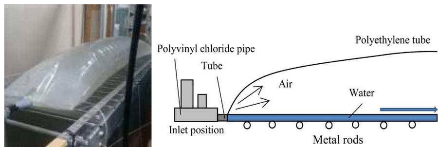
**Figure 9.** Appearance of the polyethylene tube with air injection (L: image; R: diagram).
