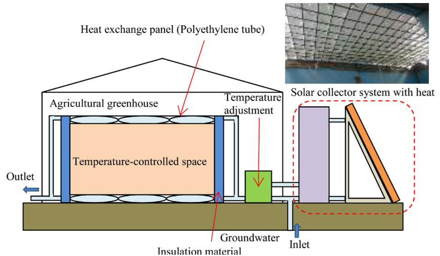
**Figure 1.** Structure of temperature control system.
