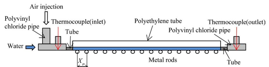
**Figure 5.** Structure of the test section.
