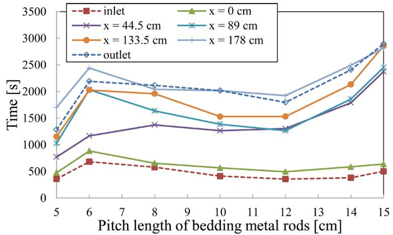
Figure 12. Relationship between time required to reach steady state and  $X_p$  with air injection.
