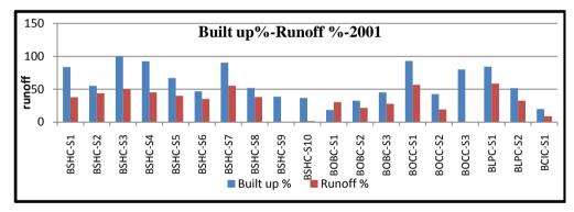
Figure 9. Build up and runoff in catchments for 2001.
