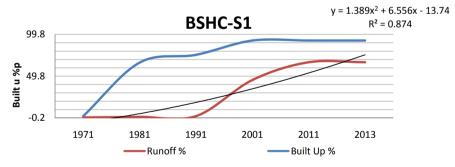
Figure 13. Build up and runoff variation in catchment BSHC-S1.
