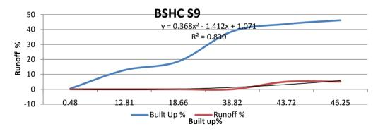
Figure 17. Build up and runoff variation in catchment BSHC-S9.
