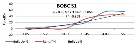
Figure 15. Build up and runoff variation in catchment BIBC-S1.
