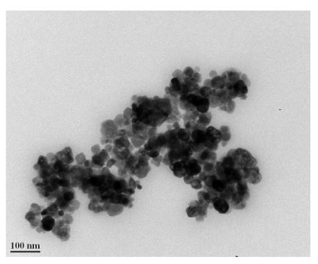
Figure 2. TEM photomicrograph of the 30 nm hematite particles. The scale bar is 100 nm. The darker areas in the image are merely caused by some nanoparticles overlying one another.
