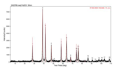
Figure 1. X-ray diffraction spectra of the spherical 30 nm hematite particles. The black line trace shows the observed spectra and the red vertical lines indicate the expected peaks for hematite.
