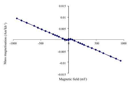
Figure 5. Magnetic hysteresis curve of the 40 nm hematite nanoparticles dilutely dispersed in water. Note the "kink" in the curve at low applied magnetic fields, which is due to the hematite nanoparticles (and which is not seen in the pure water signal of Figure 4).
