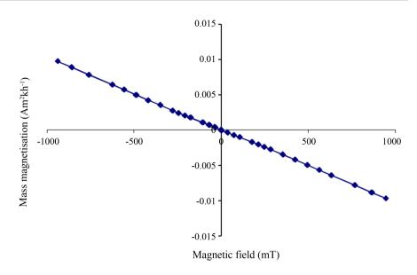
Figure 4. Magnetic hysteresis curve of the diamagnetic water that was used to dilutely disperse the 8 nm and 40 nm hematite nanoparticles.
