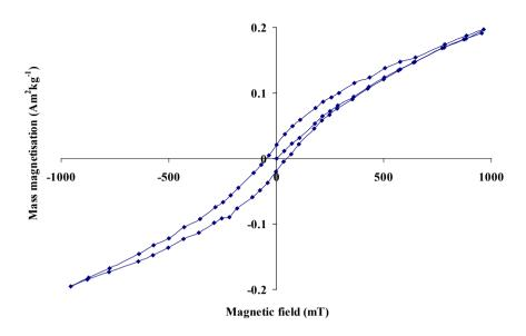
Figure 3. Magnetic hysteresis loop of the 30 nm hematite particles dispersed in calcium fluoride.
