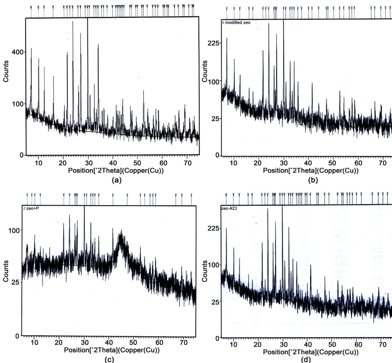
**Figure 1.** XRD of the subsequent materials (a) natural Zeolite and (b) surfactant modified Zeolite (c) Zeolite Incorporated with  $\text{KH}_2\text{PO}_4$  and (d) Zeolite Incorporated with KCl.
