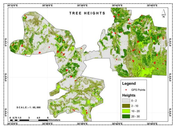
Figure 5. Canopy Heights (m), red dots represent GPS Points.
