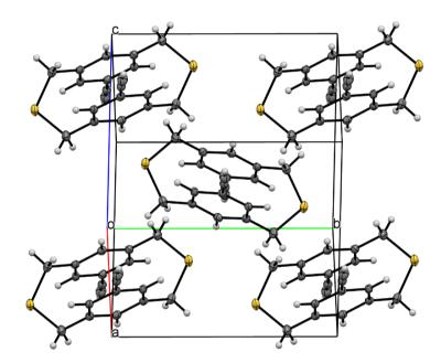
**Figure 2.** Crystal packing of 6,15-diethynyl-2,11-dithia[3.3]metabenzenophane **2a**. The yellow ellipsoids represent S atoms.
