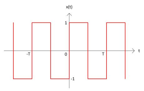
Figure 3. Square wave with fifty percent duty cycle and zero volt DC offset.
