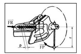
Figure 6. Work done by turning a crank.
