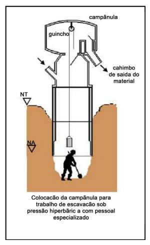
Figure 7. Work done by excavation.
