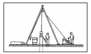
Figure 5. Work done dropping weights on piles.
