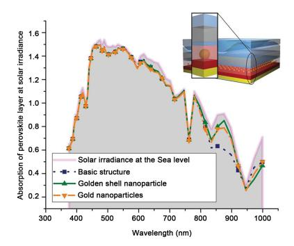
**Figure 5.** Absorption in the perovskite layer for several variants of our solar cell (basic structure, the structure enhanced by solid nanospheres, and that enhanced by nanoshells) taking into account the solar irradiance spectrum.
