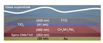
**Figure 1.** Schematics of the practical heterojunction configuration of a high-efficiency perovskite-based solar cell in accordance to [7]. The anti-reflecting coating on top of the superstrate is not shown.
