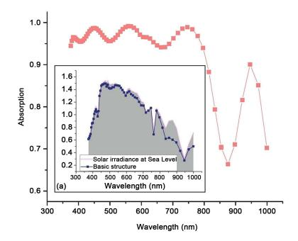
**Figure 2.** Absorption coefficient of the perovskite layer in the structure shown in **Figure 1** versus wavelength. In the inset (a) we show the solar spectrum AM 1.0 in arbitrary units (shadowed) and the spectrum of absorption in the perovskite layer.
