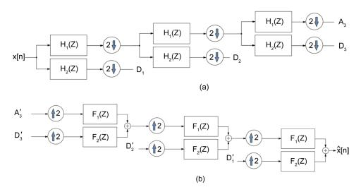
Figure 2. 3-level wavelet implementation. (a) Decomposition; (b) Reconstruction.
