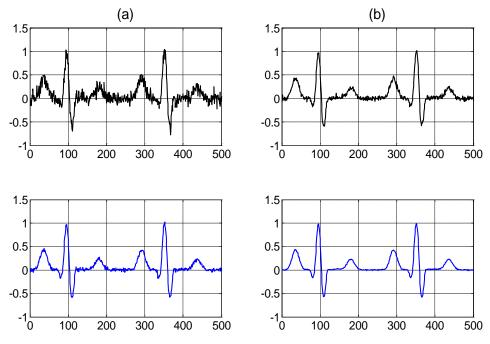
**Figure 3.** (a) The noisy and de-noised signal using proposed method (input SNR = 36.7 dB and output SNR = 48.7 dB) and (b) noisy and de-noised signal using proposed method (input SNR = 45.2 dB and output SNR = 59.2 dB).
