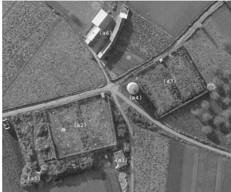
**Figure 21.** Ville Besnard logistic base on 1948—(a1) lonely bunker, modified version of R625 or R640 bunker, (a2) area with two water cisterns of German construction and surveillance post near the entrance on the road, (a3) area with two water cisterns of German construction and surveillance post on the road (a4) water tower, (a5) R630 bunker now on the site of a transmission center of Antenne Orange, (a6) farm
