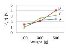
**Figure 6.** The dependence of the weight loaded on the rubber sheet sensor on the output voltage *V*<sub>o</sub>. The signs A, B and C refer to Sample A, B and C, respectively.
