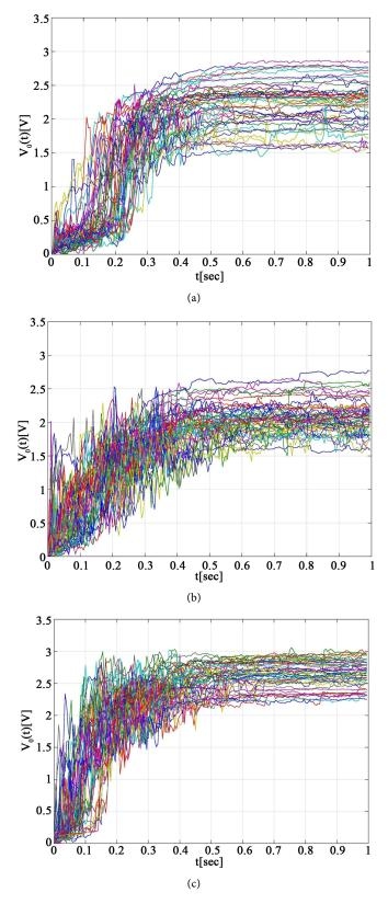
**Figure 3.** (a) The time response of the output voltage: 300 g, sample A; (b) The time response of the output voltage: 300 g, sample B; (c) The time response of the output voltage: 300g, sample C.
