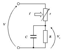
Figure 1. The detective circuit for the rubber sheet sensor (*r*).
