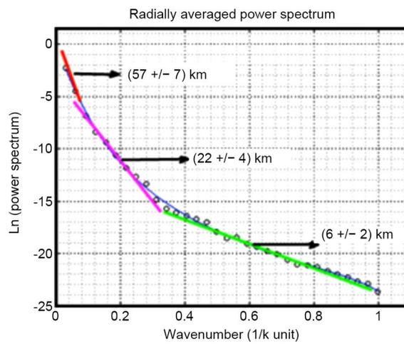
**Figure 13.** Power spectrum versus frequency for profile  $P_2$  (Kumba region).
