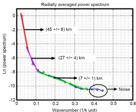
**Figure 18.** Power spectrum versus frequency for profile  $P_7$  (Ngambe region).
