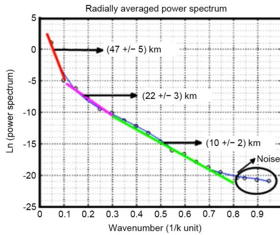
**Figure 12.** Power spectrum versus frequency for profile  $P_1$  (Mount Cameroon).
