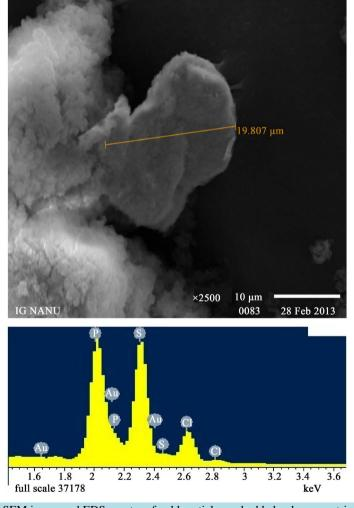
Figure 3. SEM image and EDS spectra of gold particles embedded polymer matrix.
