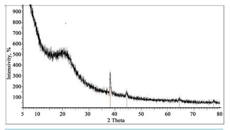
Figure 2. X-ray diffraction pattern of nanogold embedded polymer matrix.
