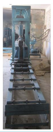
Figure 2. Mechanized system for casting of clay beams.
