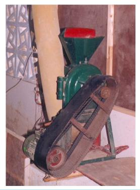
Figure 1. Clay, obtained from the quarry containing lumps, is ground in Pulverizer.
