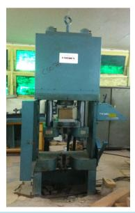
Figure 5. Baked clay cubes of 150 mm size are being tested in Universal Testing Machine.
