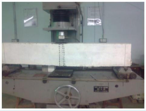
Figure 6. A white washed reinforced baked clay beam is being tested using Torsee's beam testing machine.
