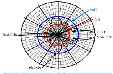
Figure 3. Typical radiation pattern of directional antenna.
