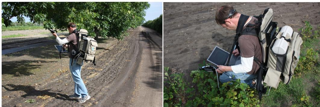
**Figure 1.** Leaf reflectance measurements using FieldSpec® Pro with leaf clip assembly for mature trees (left) and seedlings (right).
