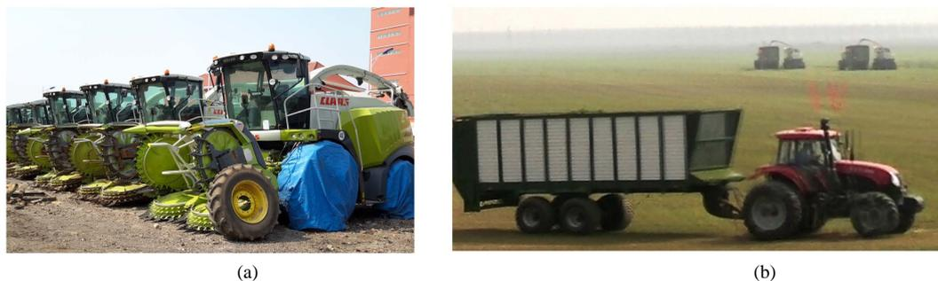
**Figure 1.** Farm machinery for forage harvesting of Huishan. (a) shows forage harvester; (b) shows forage transportation truck. Forage transportation truck which moves forages from field to dairy farm.
