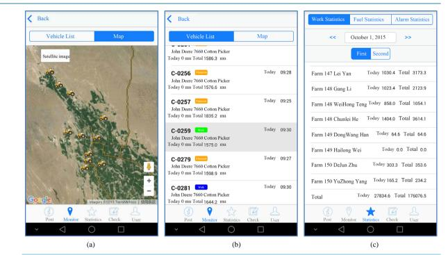
Figure 10. APP for smartphone. (a) Shows monitoring interface; (b) Shows progress of machine unit; (c) Shows progress of machine fleet.
